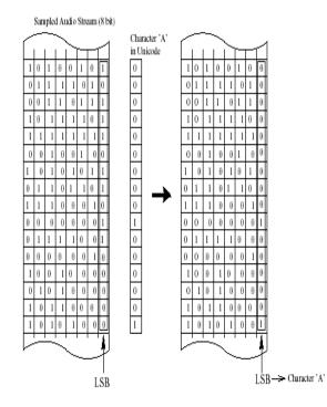
Fig 1: LSB encoding
